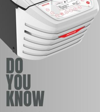
Preset feature of quick cooling mode – Rotor chamber attains 4°C from ambient temperature in quick 16 minutes
